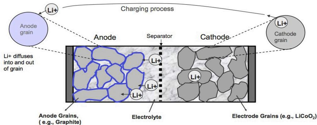
**Figure 1:** Illustration of the basic structure and operation of a lithium-ion battery. During charging, lithium ions move from the cathode to the anode, and are physically intercalated within the material grains of the anode. Graphite (carbon) is nearly universal for anodes. Cathode materials are usually made of a complex metal oxide, with Lithium Cobalt Oxide (LiCoO<sub>2</sub>) commonly used for mobile and consumer devices.
