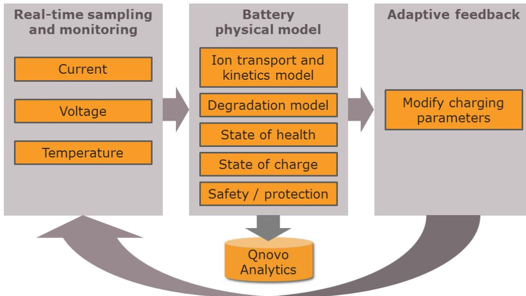
**Figure 7:** An illustration of the basic elements of Qnovo’s algorithms. The diagnostics require sampling the current, voltage and temperature of the battery. No modification of the battery is required. A model of the battery performs the requisite analysis of the diagnostics data; modulating the amplitude and timing of the pulses in the charging signal closes the feedback loop.
