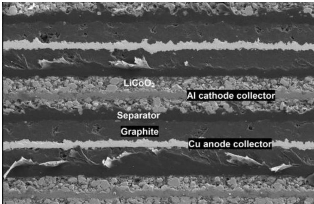
**Figure 2:** An electron microscope photograph of the alternating layers of a battery. The layers are typically 10 to 50 micrometers each. The granular nature of the layers is visible. The capacity of the battery is determined by the available material amount of anode and cathode. Battery manufacturers coat the electrode materials over large surface areas to increase the battery capacity to usable levels. Courtesy: *TechInsights*.
