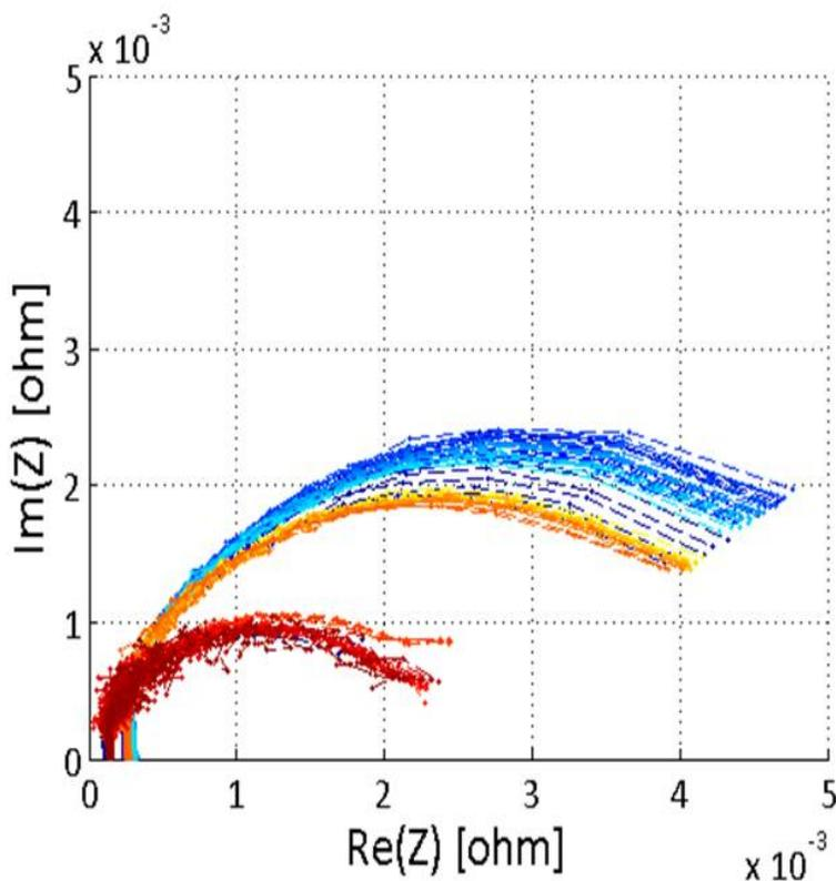
**Figure 6:** Qnovo algorithms reconstruct *in situ* the EIS graph of a mobile smartphone battery. The semi-circular curves display the real and imaginary components of the battery impedance over a range of frequencies, in this particular case, spanning from 10 Hz to 10 kHz, representing a number of processes including ion kinetics and growth of the SEI layer.
