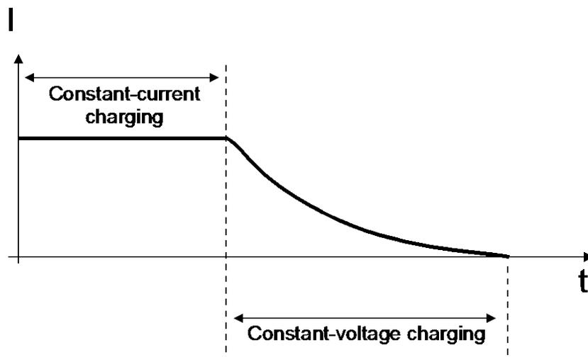
**Figure 3:** CCCV charging consists of a sequence of two steps: (i) *constant current*, during which the battery voltage rises, and (ii) *constant voltage*, after the battery reaches a predetermined maximum voltage.
